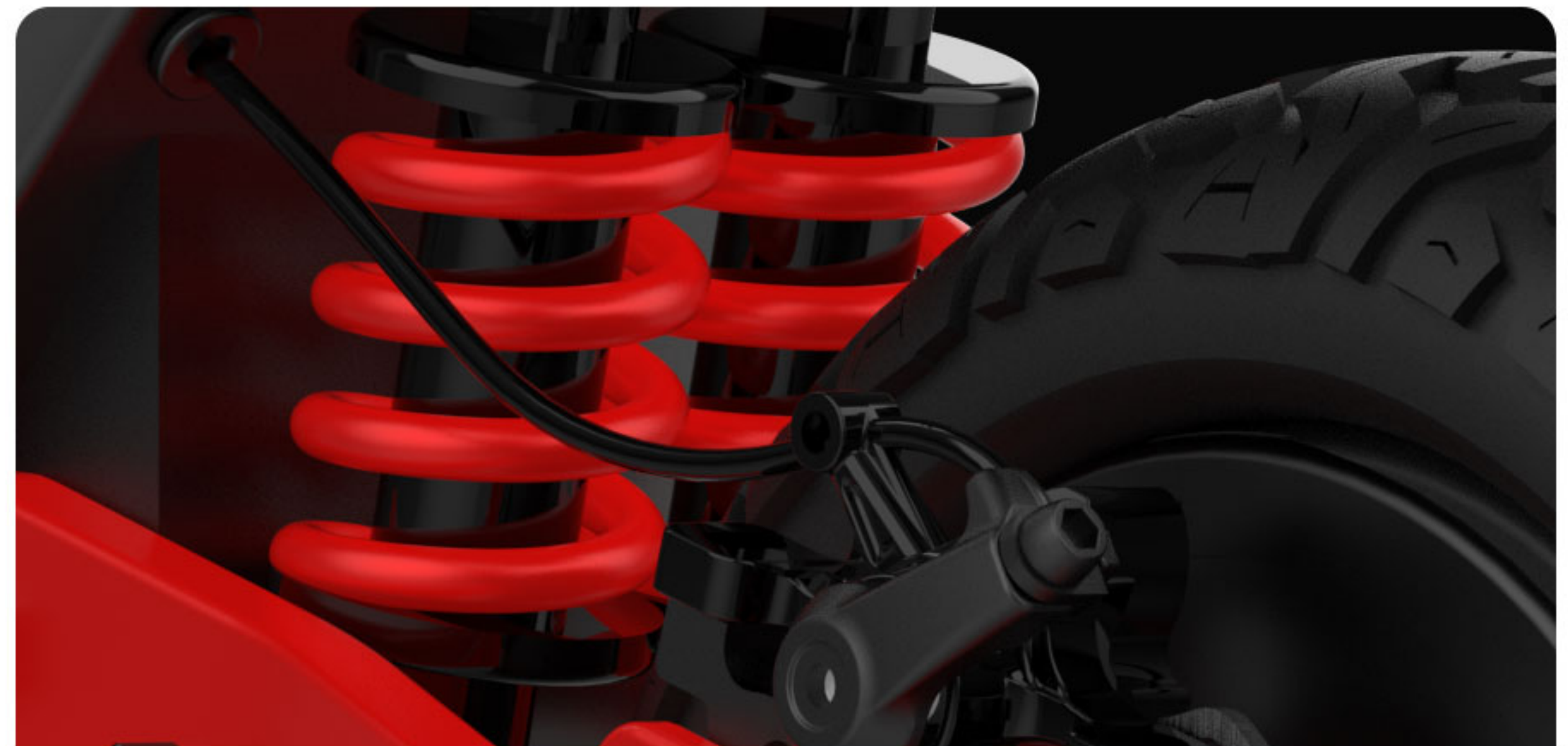
Rear dual spring damping system
